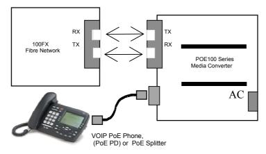
Fig. 3 POE100 Series to PD Device or POE Splitter (VOIP Phone)
