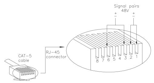
Fig. 6 Pairs used for transmitting power over Ethernet Cable.
