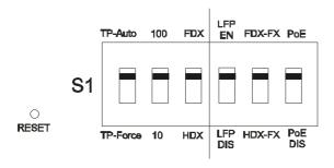
Fig. 10 Reset button and S1 – Bit 1, 2, 3, 4, 5, 6, Configuration and Settings
