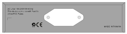
Fig. 5 POE100 Series Media Converter Rear Panel
