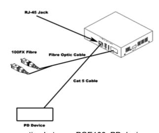
Fig. 2 Example connection between POE100, PD device and Fibre Cable
